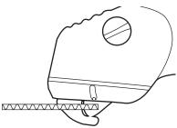
Move knife along cutting line. As knife is removed from material, Vari-Guard will spring back into position, protecting user from any blade surface.
