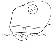
Push down until front face of knife is in full contact with material. At this point the Vari-Guard will be fully retracted, exposing straight blade.
