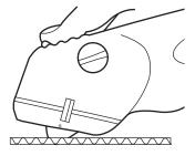
Start with knife horizontal to material. Puncture with hook blade.
